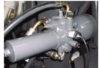
Low Pressure Filter Block For pilot circuit in the hydrostatic drive.
